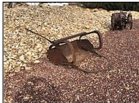
This is a Fresno, which was used to make roads.
