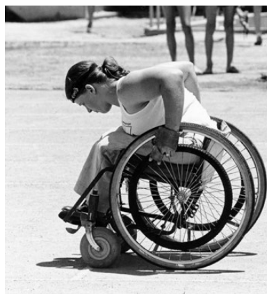
Athletics 1979 – The front wheels are still small and close to the back wheels. (P00095, Russell Collection)
