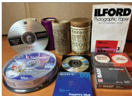
Data/Video/Audio/Image storage mediums past and present. Wax Cylinder, Cassette and Digital Audio Tape (DAT), Mini-Disc, CD-R, Mini CD-R, Blu-Ray Disc. Photographic Film. (Image courtesy of the author)
