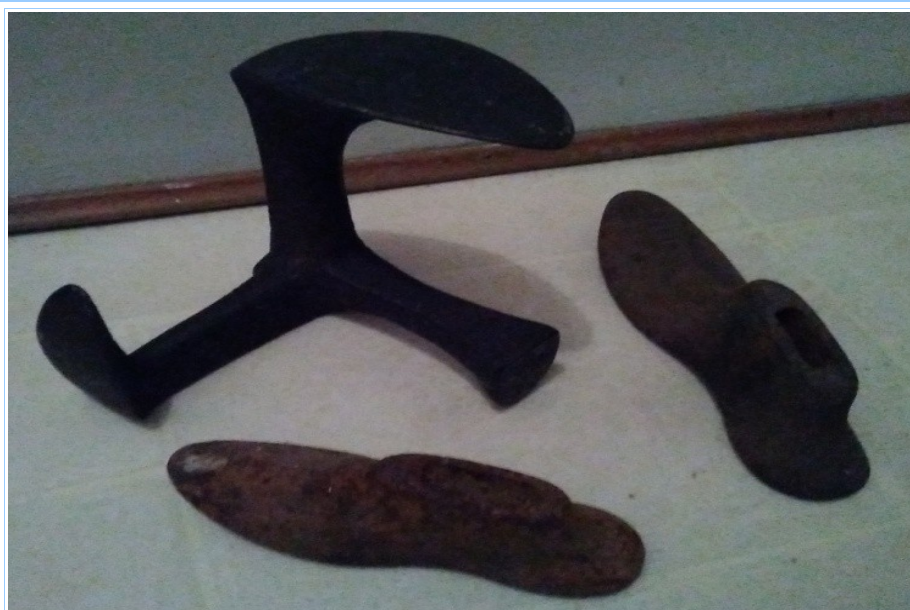
This pair of "lasts" is an original one that he made shoes on.
